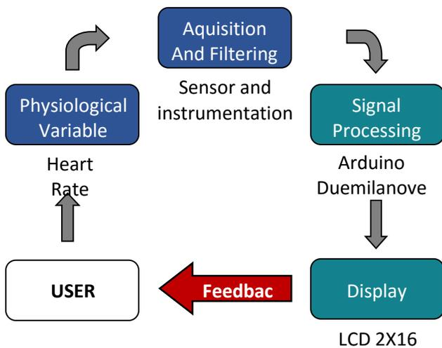
**Figure 1:** Block diagram of the proposed biofeedback system.
