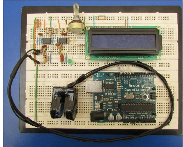
**Figure 3:** Biofeedback prototype implemented on a breadboard.
