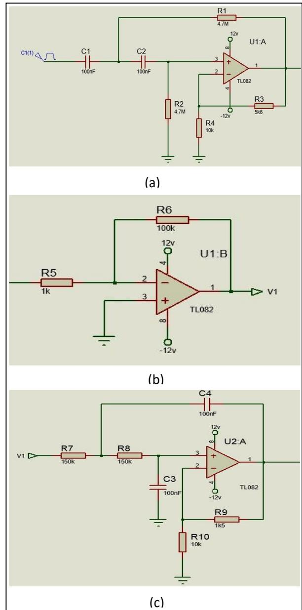
**Figure 2:** Filtering Stage: High pass filter (2(a)). Inverter amplifier (2(b)). Fourth order low pass filter (cascade of two second order filters) (2(c)).
