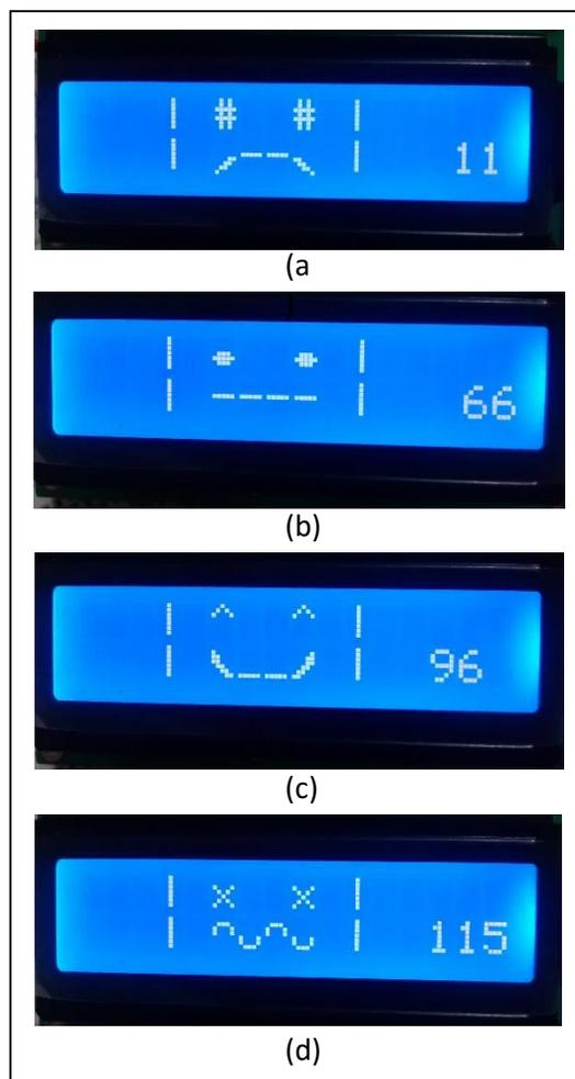
**Figure 4:** Visual feedback using mood faces for low (4(a)), medium low (4(b)), medium-high (4(c)) and high (4(d)) level of heart rate.
