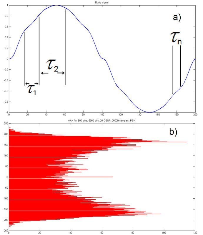
Fig. 2. a) Basic Signal b) Example AAH for 500 bins, 5000 bits, 20dB OSNR, 20000 samples and PSK modulation
