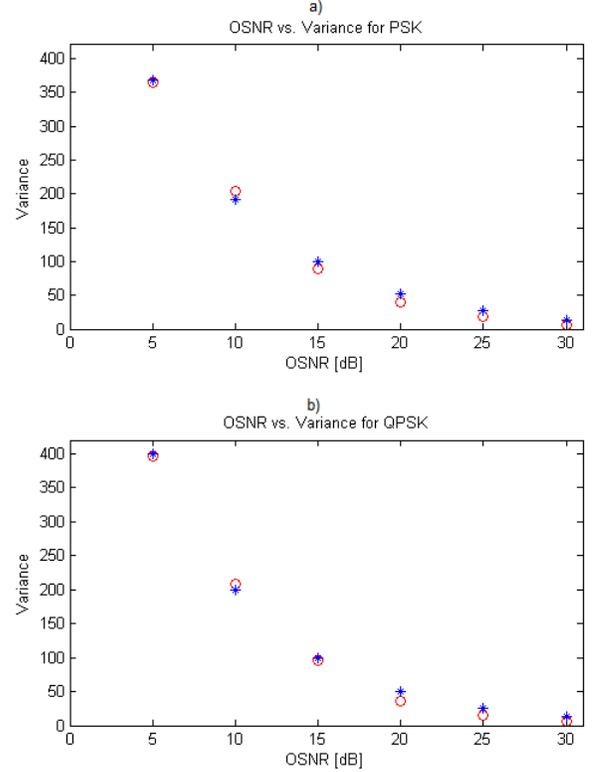
Fig. 6. Variance vs. OSNR (red circles) and the corresponding fit (blue stars) for a) PSK, b) QPSK
