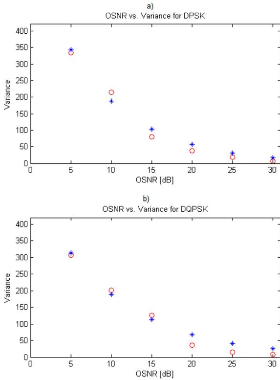
Fig. 7. Variance vs. OSNR (red circles) and the corresponding fit (blue stars) for a) DPSK, b) DQPSK
