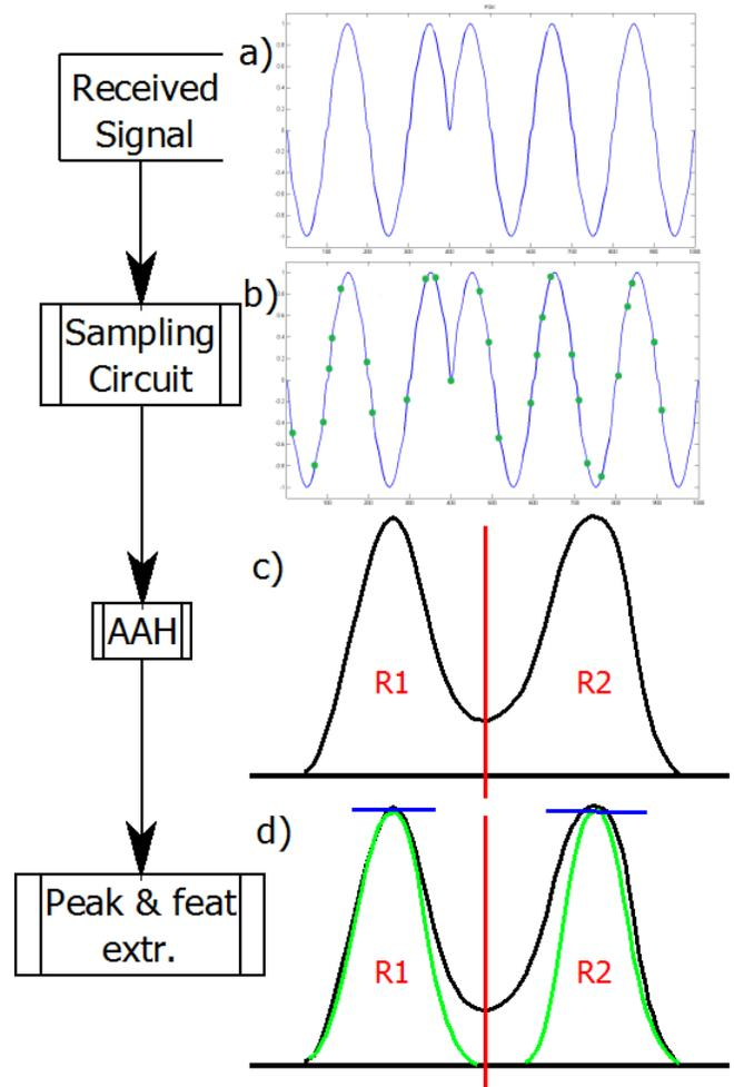
Fig. 8. Proposed OMS broken down into phases.
